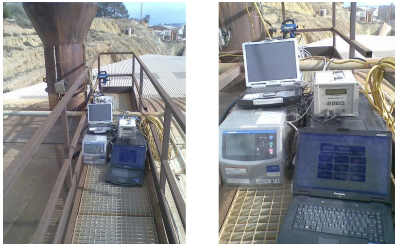
Figure 7. Equipment used during continuous monitoring of the HF emissions.
