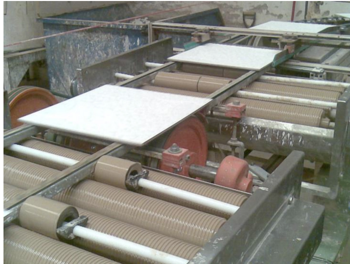
Figure 5. Coating application prototype based on the use of rollers and used during the industrial trials.
